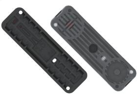
ND emitters eliminate drainage and refill effect, and improve efficiency in pulse irrigation. In order to achieve the ND function, the emitter opens at 0,40 bar and closes at 0,25 bar.
